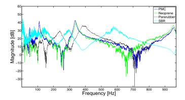
Figure 9.5: FRFs of the complete setup for different pad materials for pad width of  $5~\mathrm{mm}$
