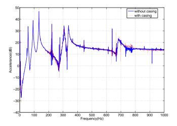
Figure 8.13: Modal analysis results with and without casing
