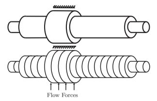
Figure 6.2: Flow forces applied to structure model (up: rotor and casing, down: meshed rotor with finite elements)
