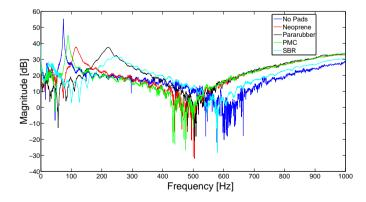
Figure 9.3: FRFs of the experiments on the support for different pad materials for pad width of 5 mm
