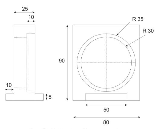
Figure C.1: The dimensions of the extra support in mm
