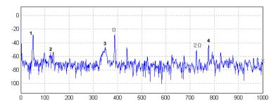
Figure 9.9: Spectrum plot at 24 900 rpm of the setup with PMC pads of 5 mm, vertical axis: db horizontal axis: Hz
