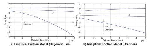
Figure 8.19: Onset of instability with different friction models-support beam length: 80 mm
