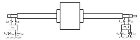
Figure 8.11: Support Model with Rotational DOF
