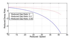
Figure 6.9: The effect of air gap on stability
