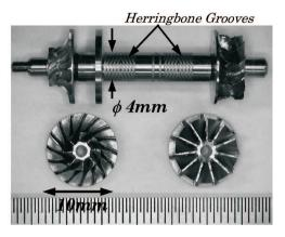
Figure 2.5: Rotor of the turbocharger [41]
