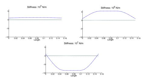
Figure 7.3: Mode shapes for the first natural frequency at different support stiffnesses
