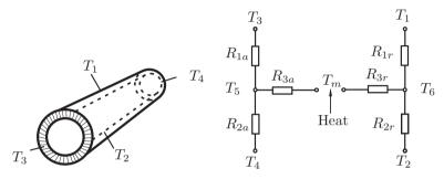
Figure 5.1: Thermal networks for a cylindrical section [54]
