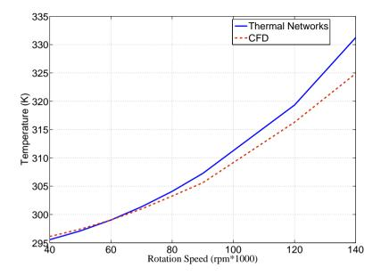
Figure 8.23: Thermal Network and CFD Results
