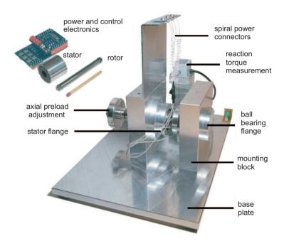
Figure 2.7: Ultra-high-speed test bench with motor in the right flange and generator in the left flange [92]
