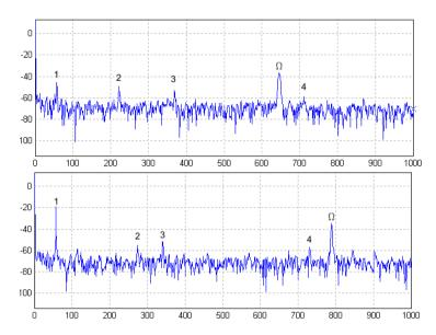
Figure 9.14: Spectrum plot at 40 000 (above) and 49 900 rpm (below) of the setup
