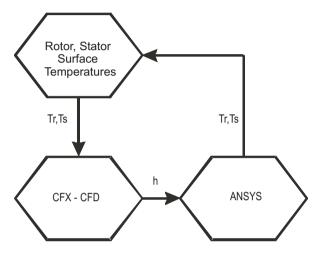
Figure 8.20: ANSYS-CFX Coupled Thermal Analysis Procedure
