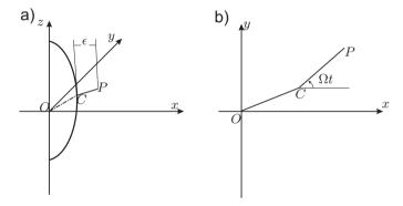
Figure 3.4: Unbalanced rotor a) sketch of the deflected system b) situation in the xy plane [32]
