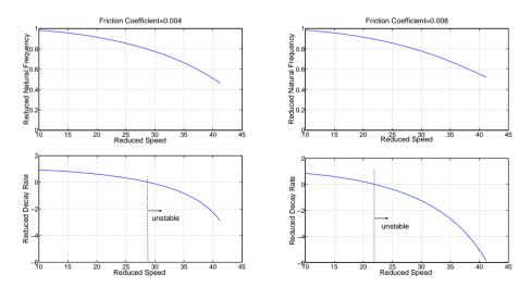
Figure 6.7: Change of first natural frequency and decay rate with friction coefficient
