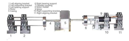
Figure 7.8: The complete experimental setup
