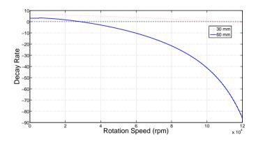
Figure 7.2: Decay rates for disk diameter of 60 mm and 30 mm
