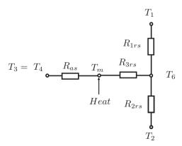
Figure B.1: Thermal network for a symmetric cylindrical section [54]
