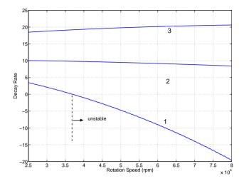
Figure 8.17: Theoretical prediction of onset of instability-support beam length: 80 mm
