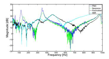
Figure 9.6: FRFs of the complete setup for different pad materials for pad width of 10 mm
