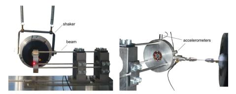
Figure 8.5: Modal analysis of the isolated support
