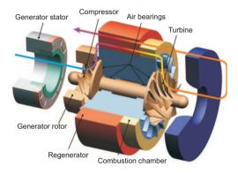
Figure 2.3: Initial Design of the microturbine in Belgian Power MEMS Project [60]
