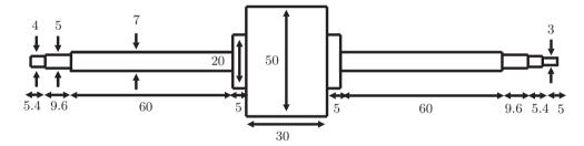
Figure 7.4: The dimensions of the rotor
