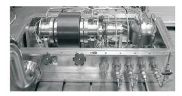
Figure 2.6: Horizontal axle type flywheel [75]
