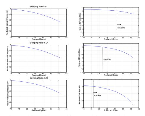
Figure 6.6: Change of first natural frequency and decay rate with damping
