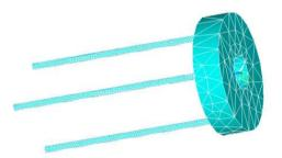
Figure 7.7: ANSYS model of the support
