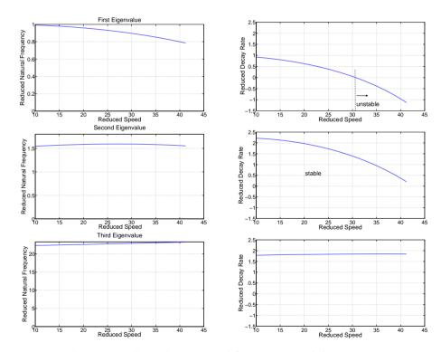
Figure 6.4: First three natural frequencies and decay rates
