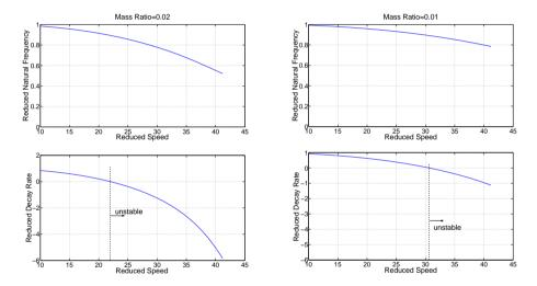
Figure 6.5: Change of first natural frequency and decay rate with different mass ratios
