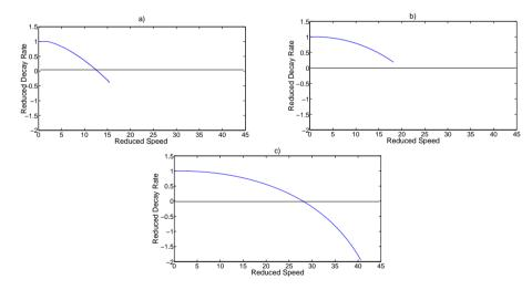
Figure 7.10: The reduced decay rate for different applications: a) The experimental setup b) Microgenerator, support stiffness:  $5 \times 10^4$  N/m c) Microgenerator support stiffness:  $1 \times 10^4$  N/m
