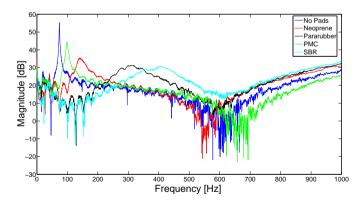
Figure 9.4: FRFs of the experiments on the support for different pad materials for pad width of 10 mm
