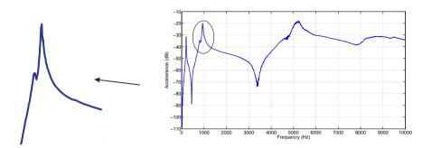
Figure 8.7: FRF of the rotor with rigid supports
