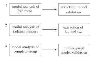
Figure 8.2: Experimental procedure
