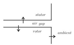
Figure 5.3: The convective heat transfer directions
