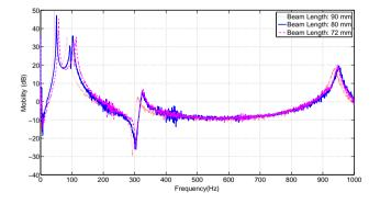
Figure 8.9: Modal analysis results with different beam lengths
