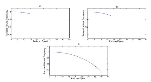
Figure 7.9: The reduced natural frequencies for different applications: a) The experimental setup b) Microgenerator, support stiffness:  $5 \times 10^4$  c) Microgenerator support stiffness:  $1 \times 10^4$
