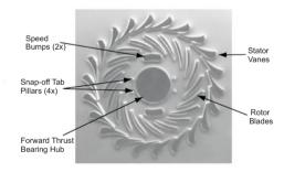
Figure 2.2: Optical photograph of the 4.2-mm diameter microturbine showing the stator and rotor blades [29]
