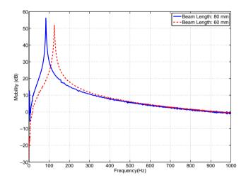
Figure 8.6: FRFs of the support with different beam lengths
