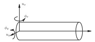
Figure 3.1: Beam element
