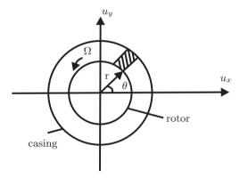
Figure 4.3: Two dimensional annular flow
