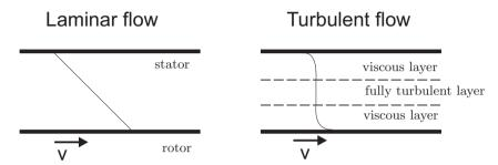
Figure 4.1: Tangential velocity profiles of laminar and turbulent air gap flows [67]
