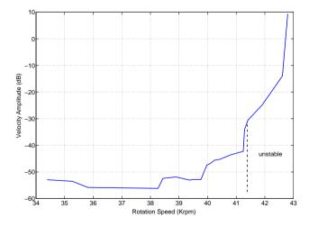
Figure 8.16: Amplitude of velocity spectrum at different rotor speeds
