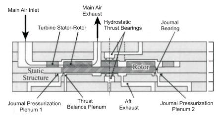
Figure 2.1: Schematic of a cross section of the microturbine-driven bearing rig. For scale reference, the rotor is 4.2 mm in diameter [29]
