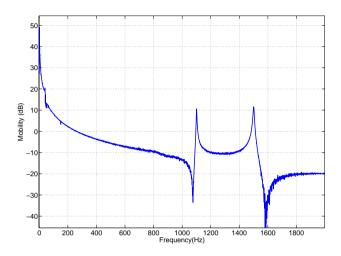
Figure 8.4: Frequency response function of the free rotor
